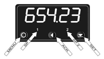
The key **MENU** opens the program menu. The required parameter will be confirmed with **ACK**. The parameter magnitude will be set with **ACK** or **SET**.
