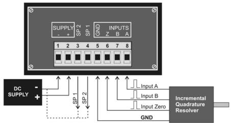
SP1 and SP2 are open collectors, optocoupler type PC 357. The emitters are internally connected to (-) supply
