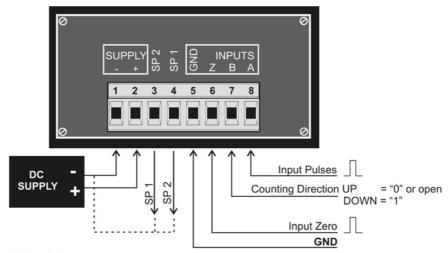
SP1 and SP2 are open collectors, optocoupler type PC 357. The emitters are internally connected to (-) supply
